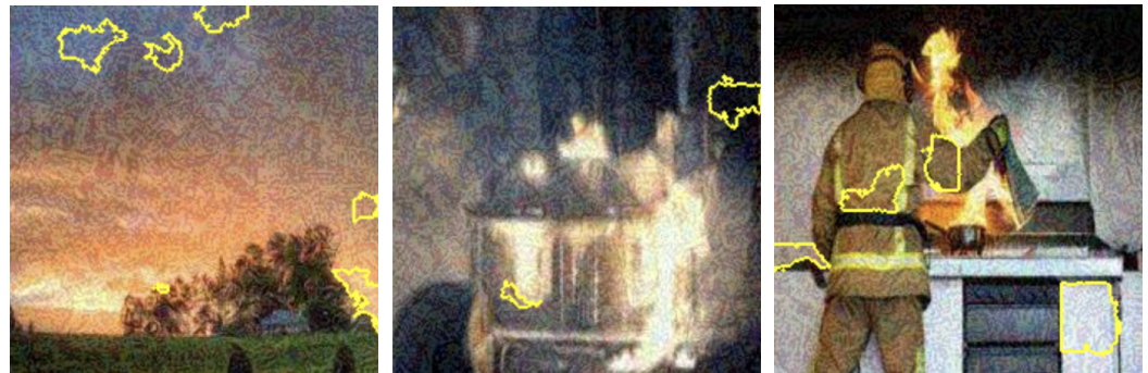
Figure 7. LIME saliency maps in RGB showing misclassifications from FGSM perturbations as focus shifts from flame regions.
